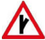
Sharp Junction Ahead, to Right Sign
