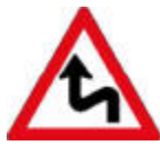
Combined Curves Ahead, First Left Sign
